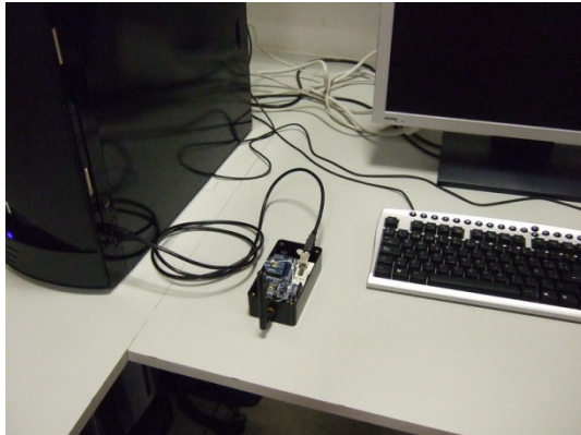
Fig. 14 Coordinator connected to a Computer USB Port in Lab 1.2
