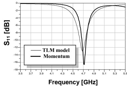
Fig. 3 Simulated input antenna return loss.
