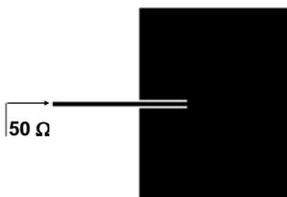
Fig. 7 The mask layout of the inset fed patch antenna design operating at 5.4 GHz. The parameters are set to:  $W_o=16.28$  mm,  $L=12.7$  mm,  $S=0.42$ mm,  $W_f=0.42$  mm,  $Y_o=4$  mm.
