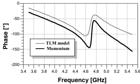
Fig. 5 Reflected phase at the antenna input.
