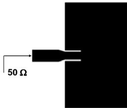
Fig. 2 The mask layout of the inset fed patch antenna design operating at 4.7GHz. The parameters are set to:  $W_a=32.4$  mm,  $L=19.3$  mm,  $H=1.27$  mm,  $S=0.57$  mm,  $W_f=2.4$  mm,  $Y_0=4.9$  mm.
