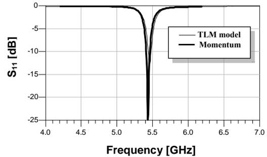
Fig. 8 Computed return loss of the inset fed antenna.
