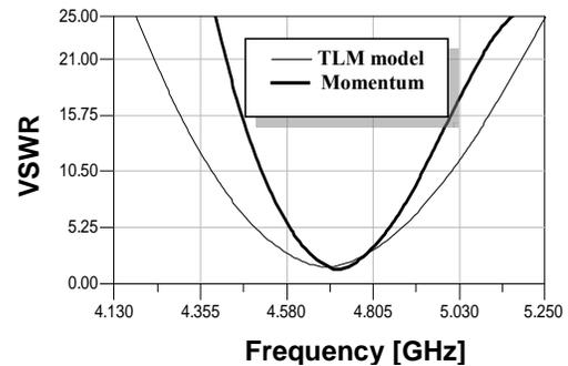
Fig. 4 Simulated input antenna VSWR.
