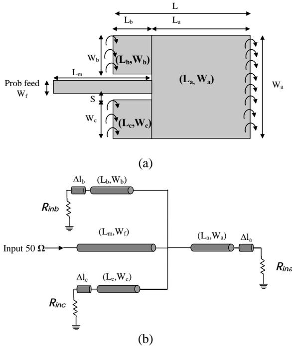
Fig. 1 (a) Inset fed antenna. (b) Equivalent circuit of the proposed antenna.
