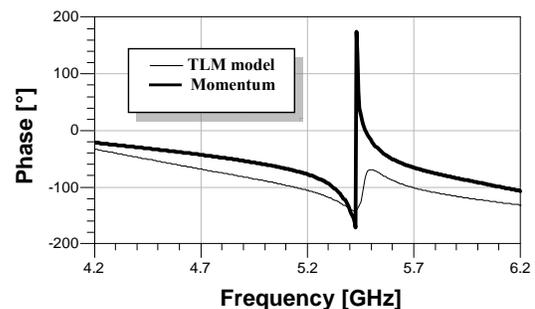
Fig. 10 Reflected phase at the antenna input.
