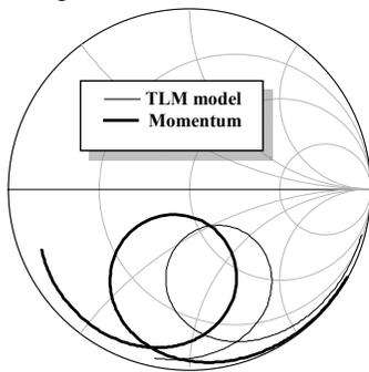
Fig. 6 Smith's chart of the input impedance return losses. Frequency points given by start = 3.3 GHz, stop = 5.4 GHz.
