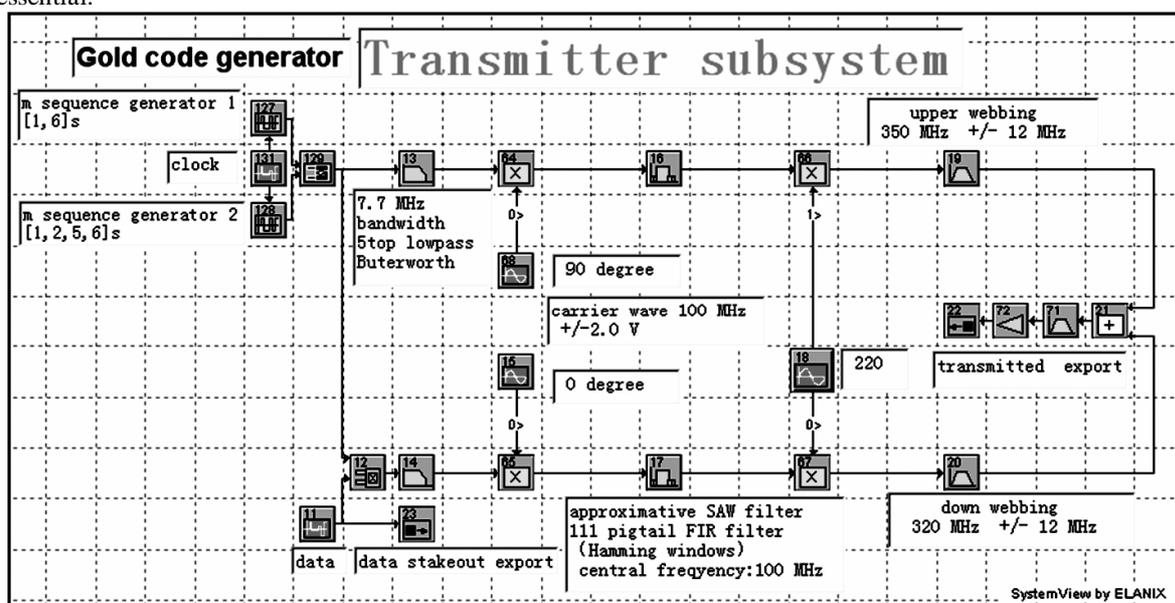
Fig. 3 Transmitter subsystem
