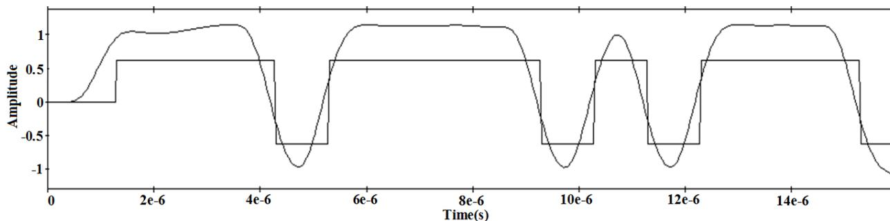
Fig. 4 The export signals add with original signals after Coatas loop demodulation
