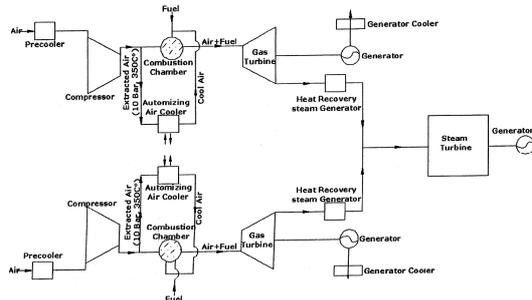
Fig. 1 Diagram for gas turbines in power plant
