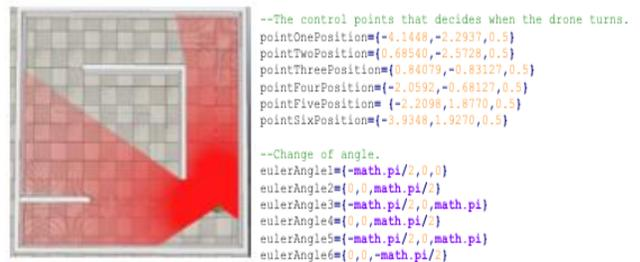
Figure 6. a) Observation area path b) The cod controlling the UAV turning 90°.
