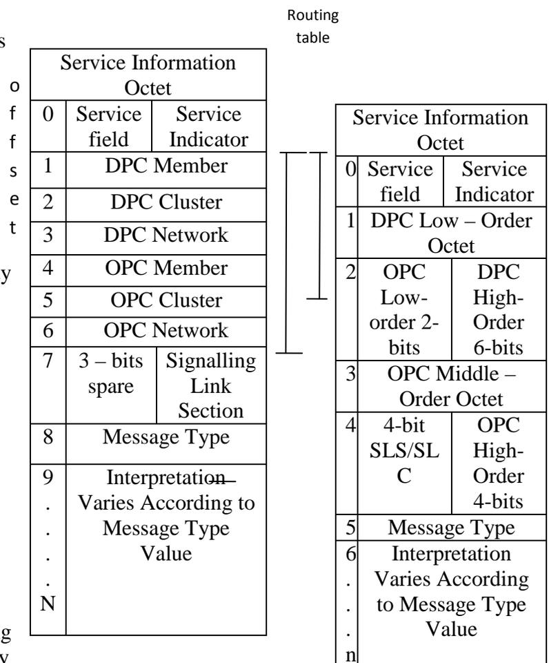
The signaling information field(SIF) contains the routing label followed by the SCCP message header with the following structure:
