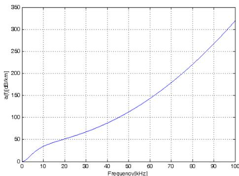
Fig. 2: Absorption coefficient  $\alpha(f)$  in frequencies less than 100 kHz.
