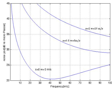
Fig. 1: Noise PSD versus frequency for 3 arbitrary selections of  $s$  and  $w$ .
