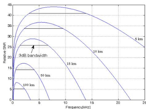
Fig. 3: Relative SNR versus Frequency in 5-100 km
