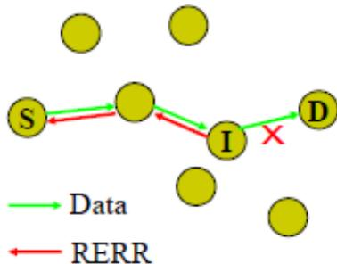
Fig 6 AODV routing protocol with RERR message
