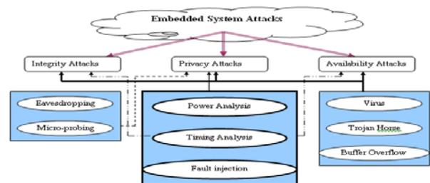
Figure 2. Embedded System attacks [6]
