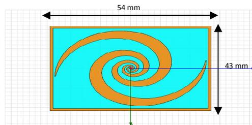
Fig.8: Design of the spiral antenna
