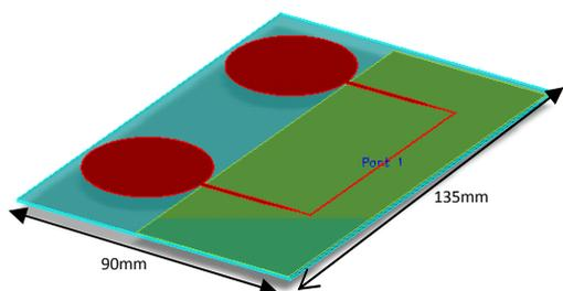
Fig.12: Array of circular patch antenna
