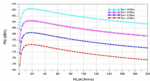
Fig.7: Variation of the DC power according to the load RL.
