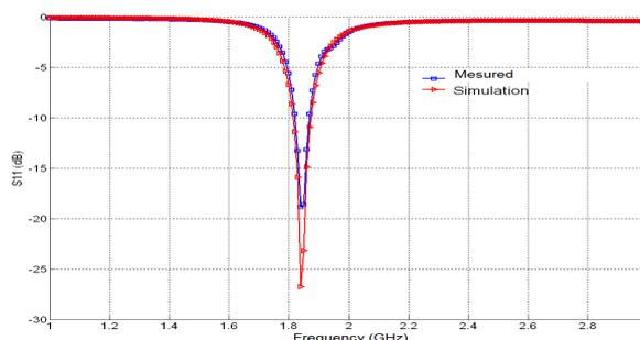
Fig.5: Variation of the return loss measured and simulated according to the frequency with  $P_{RF} = -40\text{dBm}$ .
