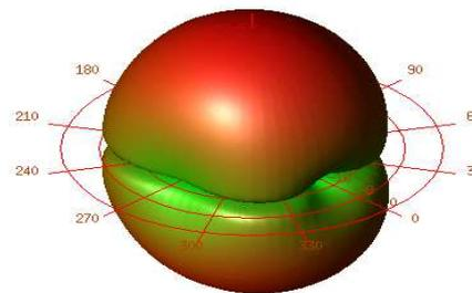
Fig.14: Radiation pattern at 1.85GHz
