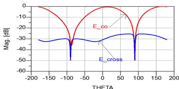
Fig.15: Polarization of the field E at the frequency at 1.85GHz
