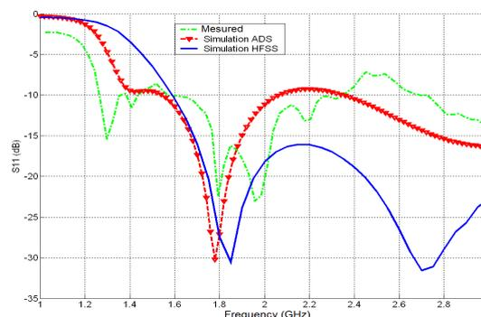
Fig.9: variation of the return loss according to the frequency.
