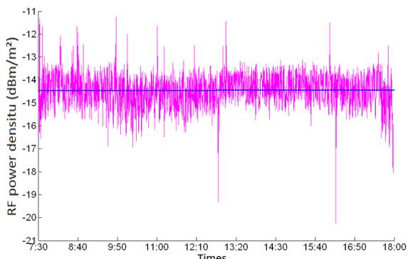
Fig.2: Variation of the total density of the power RF in the wave-band 1800MHz-1900MHz
