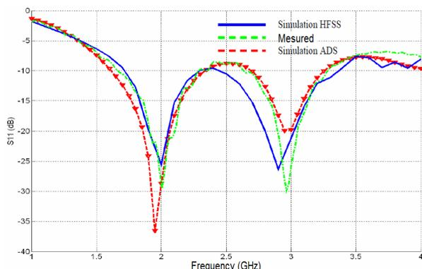
Fig.13: Variation of the return-loss according to the frequency
