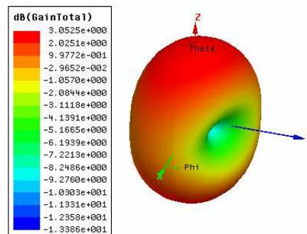
Fig.10: Radiation pattern at 1.85GHz
