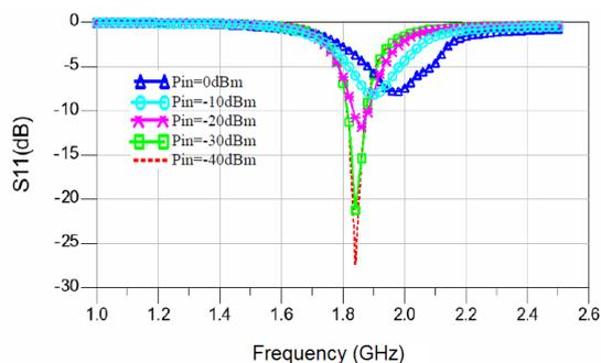
Fig.6: Variation of the return loss simulated according to the power RF.
