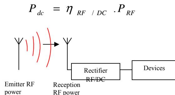
Fig.1. Conceptual view of the harvesting RF energy system
