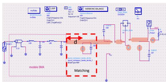
Fig.3: Circuit of the converter RF/DC
