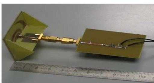
Fig.16: Prototype Of the rectenna based on a spiral antenna
