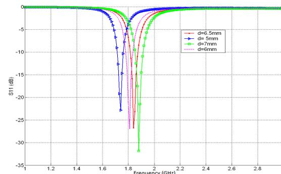
Fig.4: Variation of the return loss simulated according to the distance d.
