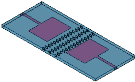
Fig. 3. 3D view of the array antenna with SR structure for 3 rows
