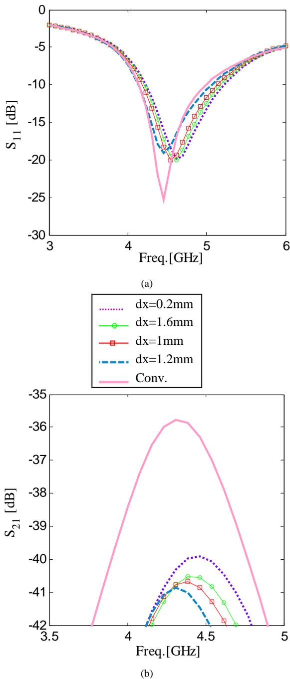
Fig. 9. Return loss (a) and mutual coupling (b) for different spacing in the X direction with 5 rows
