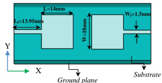
Fig. 1. Top view of two coupled microstrip antenna patches
