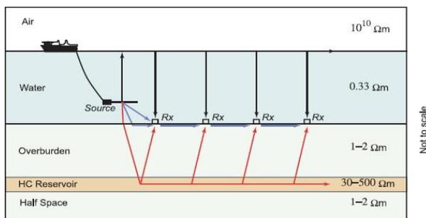
Figure 1. A Schematic diagram of Seabed logging application showing the direct waves, air waves, reflected waves and refracted waves.[11]
