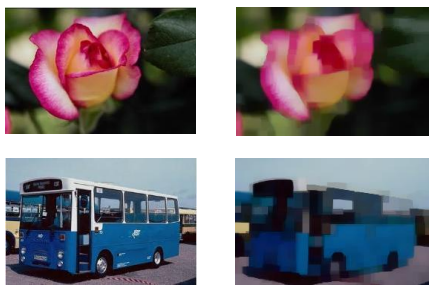
Fig. 2 The effect of morphological opening followed by closing using a 9x9 structuring element of ones.
