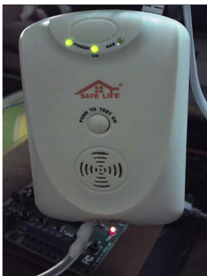
Fig. 1 The used CO alarm with air ump tube
