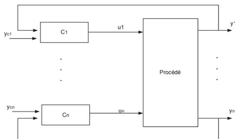
Fig. 1 Structure of decentralized control (or distributed)
