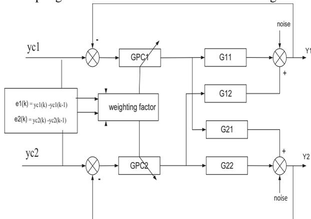
Fig. 3 Control structure of generalized predictive control with weighting factor adjusting.
