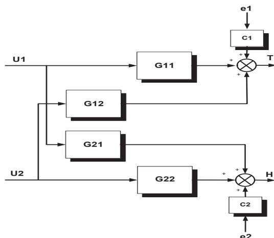
Figure 5. Input-output model of incubator system.
