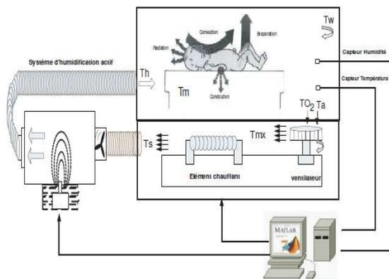
Fig. 4 Schematic of the incubator process with experimental arrangement for active humidification to control temperature and Humidity.
