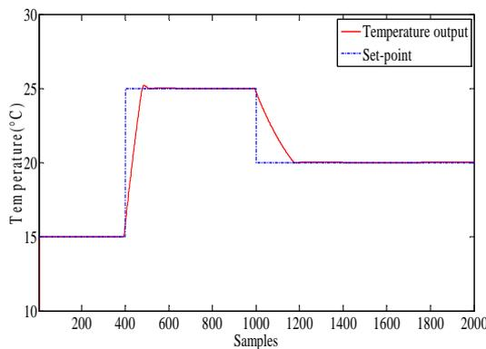
Fig. 6 Simulation result of set-point tracking temperature for predictive decoupling control.
