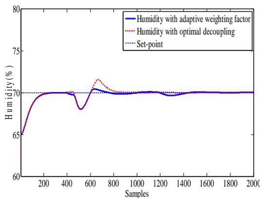
Fig. 7 Compared result of set-point tracking humidity with tuning weight factor by reference change and by adding interaction compensators
