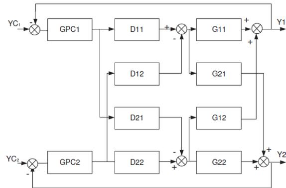
Fig. 2 Configuration of GPC decoupling control system.
