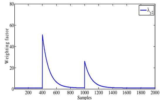
Fig. 8 Evolution of the weighting factor synchronized with change set point.
