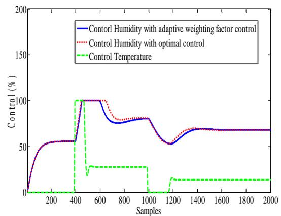
Fig. 9 Simulation results of temperature and humidity control with decoupling in incubator system
