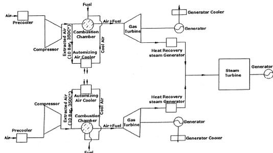
Fig. 1 Diagram for gas turbines in power plant
