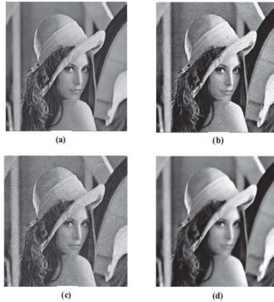
Fig.11. Performance comparison of One Dimensional and two dimensional TV denoising method with SNR 15 dB: (a) Input image; (b) is the noisy image with SNR 15 dB; (c) result of 2D TV denoising; (d) result of proposed algorithm
